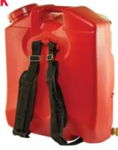
16 Litre Rigid Knapsack • Brass Plunger Pump • Adjustable Straps • Shaped for Comfort • No 8 Bushfire Nozzle • Straight Jet/Flat Fantail • Spraying Capacity 1.25lpm • Approx. 650mm tall and 495mm wide
